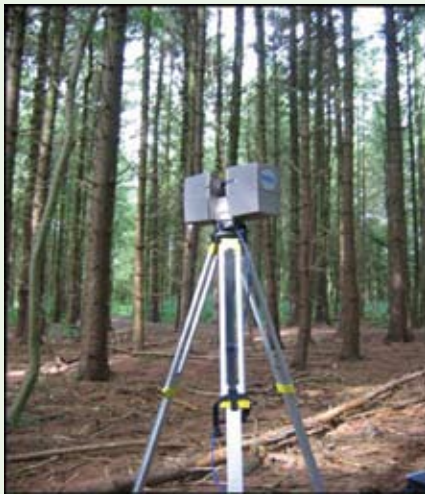
Figure 1. A terrestrial laser scanner positioned in a stand ready for a 360° scan.
